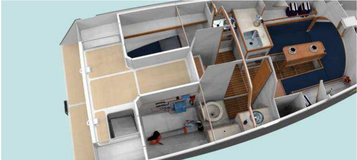
The anchor rode well is also generously proportioned, and a space for a manual windlass is provided (electric windlass could be installed for diesel powered versions or if a backup petrol generator is present).
