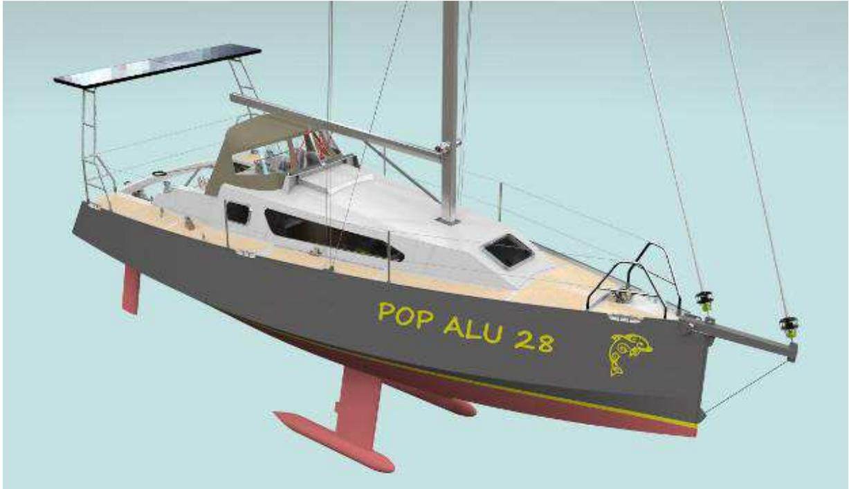
The Pop Alu 28 unites the performance orientated sail plan of the Pop 25 with the robust aluminum construction of the Pop Alu 32, offering complete CNC kits for both the aluminum structure and the interior fit out plywood panels.
