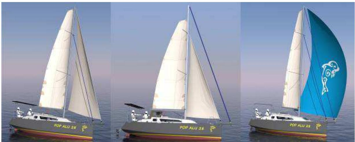
We decided to offer the Pop Alu 28 as a compact blue water, all weather cruising boat, capable of cruising the world's oceans in total safety. The design meets the criterion from the European Community for open water, being in class A according to the Monohull Stability Index (STIX).
