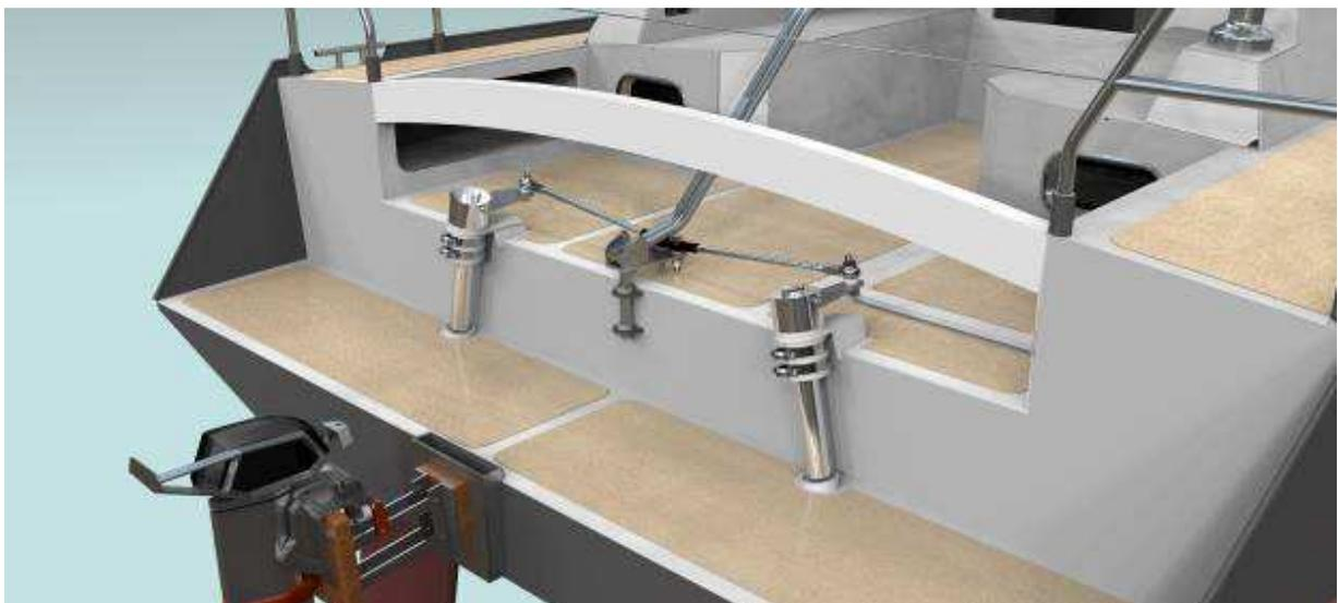
For comfort we planned a dodger and a mainsail sheet that is managed from under it, freeing the cockpit and enabling protection while in easy reach of sail controls.
