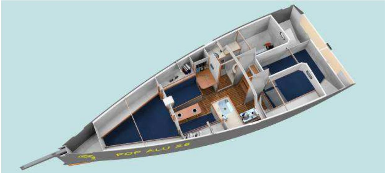
There is an aft cabin with double berth separated from the main ambient by a curtain, a double V berth forward and a comfortable saloon with 5 places, because one guest can seat in the forward bed, as we structured the mast frame in a way to obviate the need for a mast column, leaving the entrance to the forward cabin totally free.
