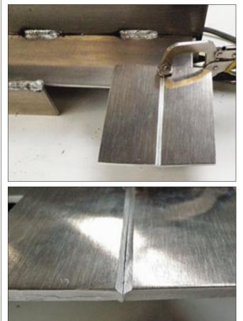
Close up view of edge preparation in readiness for butt weld. We will assume the plates are tacked on the back side for this example.
