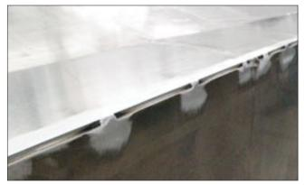
This corner has been fully welded on the inside. The outside welds are sanded down then back cut before final welding.
