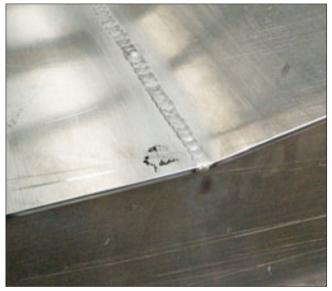
The finished welds require cleaning and external sanding if desired. After leak testing, commercial boats would be finished at this stage. On the inner chine weld we would remove the high spots, (stops and starts), and we may sand the external edge for visual appearance.
