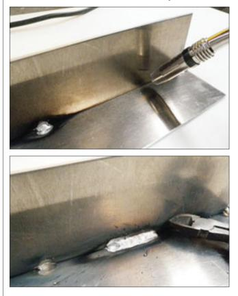
parts are intermittently stitched with a 50mm weld at 150mm spacing.
