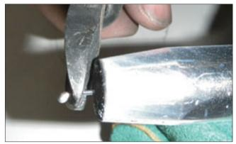
When the weld is finished, it is good practice to snip the end of the wire protruding from the MIG gun nozzle. After the welding operation, sometimes a ball appears at the end of the wire. To get a better weld start, you must remove this ball.
