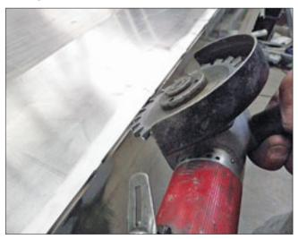
This photo shows the tool we use for back cutting. It is an air grinder with a metal cutting blade. These tools are excellent for removing large amounts of material quickly and without depositing grinding wheel material in the groove. These tools are also VERY dangerous and we would not recommend an inexperienced operator to use them.
