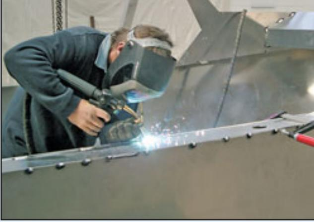
Tack two of the deck longitudinals in place. We tack these to keep the frames upright, but leave enough room to access the stringers for welding. Starting at the keel, weld intermittently the keel join, all the stringers, starting at the keel, working outwards, port to starboard, diagonally, and front to back. This zig-zag pattern of welding keeps heat build up to a minimum and will reduce the risk of distortion.
