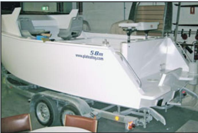
With the boat now finished it is ready for paint. The sequence we use is 2 pack etch primer, epoxy filler, epoxy undercoat then epoxy topcoat. We use International HT9000 two pack epoxy, (with micro balloons), for filling. Previous PAB articles (PAB-3 especially) have a good explanation of preparation and painting, so I will not repeat what is a great article that
