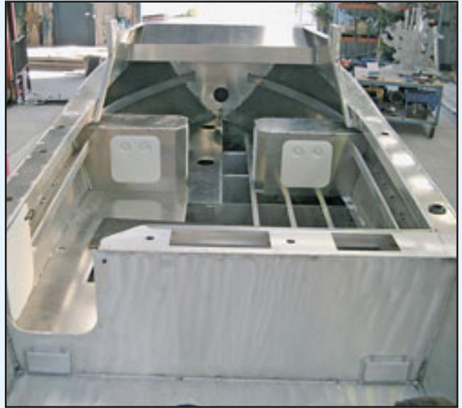
Weld all top edges, fit and weld the inner rear panels and weld on the outer coamings. The bow sprit can be fitted corner to corner and welded in place. If a bolt on bow roller is to be used it is worth tacking a scrap of 5mm to the underside to allow a little more material if tapping with screws.
