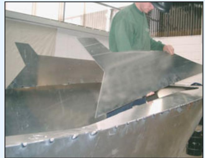
home. Fold the plate to the angle of the engraving marks on the inner cab sides and fit the dash panel and tack in place on both sides. With the dash panel fitted and the cab sides tacked on, the inner gunnel coaming can be tacked on.
