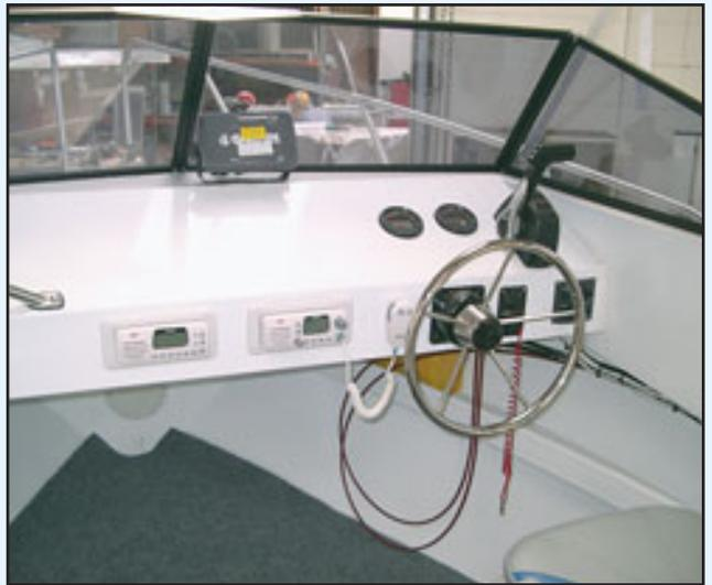
and deck wash pickup are shown. At the helm, hydraulic steering, a switch panel, marine radio and 27 MHz, Depth / GPS Combo unit and swivel / sliding seats provides a basic fit out. The fit out can be an expensive exercise, but the boat can be designed with provision to upgrade when then funds permit. Always give thought to under floor connections and or wiring before the main plates are welded in. i.e.: Is a bilge pump needed, if so, wire for power and outlet to vent.
