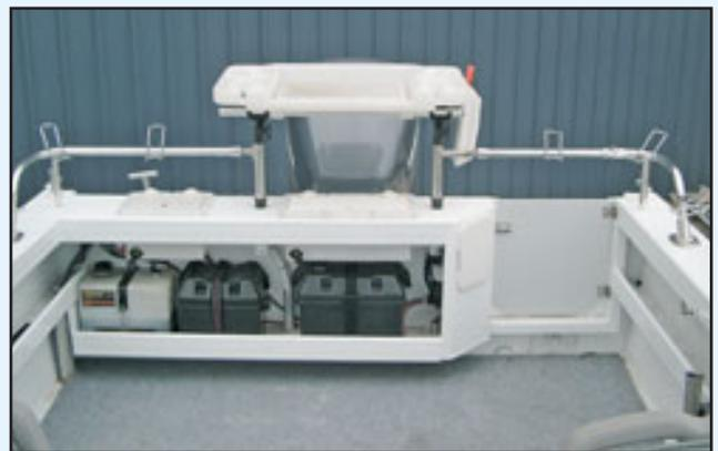
you can build in a live bait tank in the starboard rear side and still have room for 2 large batteries.
