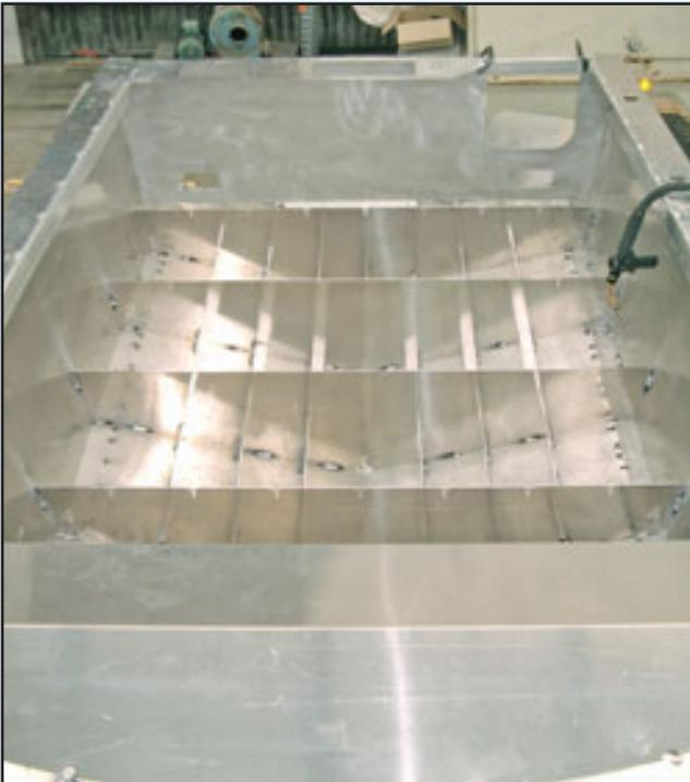
With the main external hull welds complete, and the hull leak tested, the keel coaming can be fitted. It is easiest to roll the boat over to do this. (Another BBQ, a few mates are needed, and the hull can be easily rolled over). Be sure to support the hull safely. Leave the weld proud on the keel, do not sand back, and fit the coaming around the keel edge.
