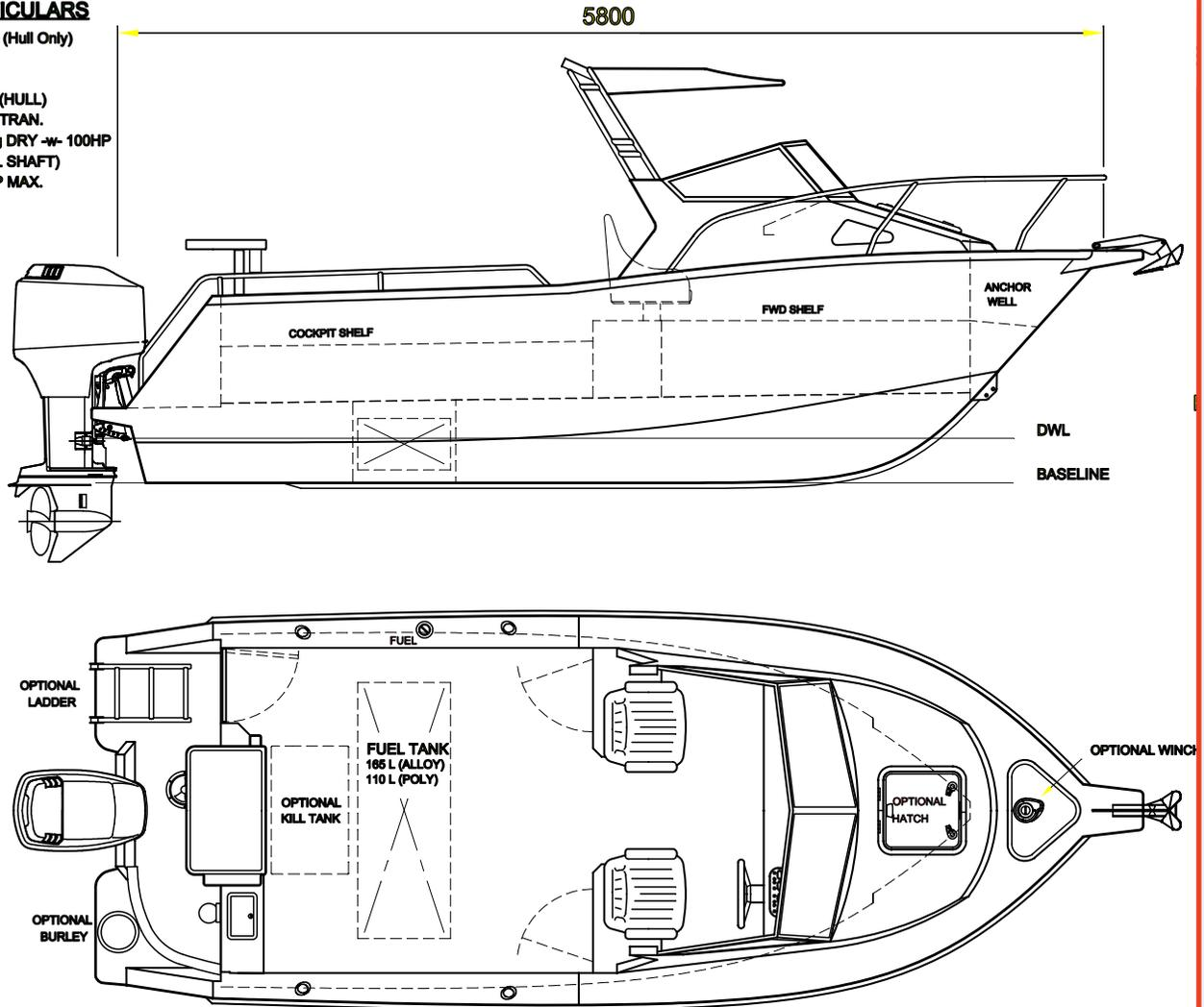
**Kit Notes: Bimini / Launcher, Ladder and Fuel Tank not included in Flat Pack Kit. Typical fitout options shown.**
