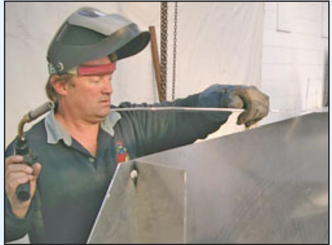
drawings, and tack a temporary brace across the boat. Next, tack the rear gunnel plates, and the rear top plate in place. We also tack a strong-back, (or stiffener) across the back of the rear panel at floor level and also where the door opening is to keep the panel straight.
