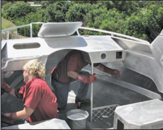
A slightly modified cockpit by a Queensland owner. Dash cutout and fabricated hatch can save \$650-. Note the grab handle on the dash and side in-fill panel for engine control, (side mount).
