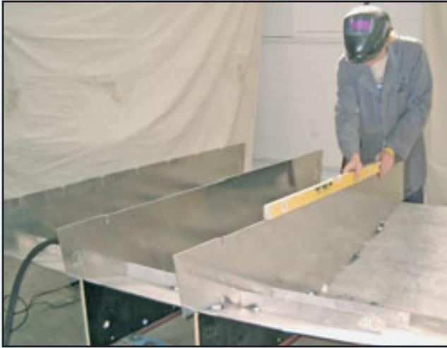
and 3 tacks on one side, and 2 tacks on the other side staggered arrangement. The stringer should be fitted so that it fits hard up against the bottom plates. In the bay where the fuel tank is fitted, we fit angle to support the fuel tank. The plates either side of the fuel tank bay are stiffened at the outsides, and also have gusset plates.
