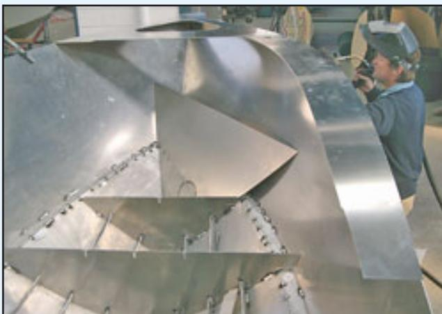
Once the side plates are tacked on, tack the front anchor plate in position, with a few small tacks. We need this in position, so we can position the forward gunnel plates, confirm the dimensions from the construction
