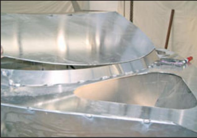
The inner chine and outer chine can be welded. We normally weld on the inside first, then back-cut the outer and get a good penetration weld on the outer chine and flush sand. The inner chine (underside), we weld and leave un-sanded. All the external welds on the hull are welded both sides.
