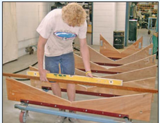
1c etc, outward toward the chine. The frame numbers are marked and are aligned with the marks on the bottom plates. These numbers are also marked on the chine and side plates for alignment.
