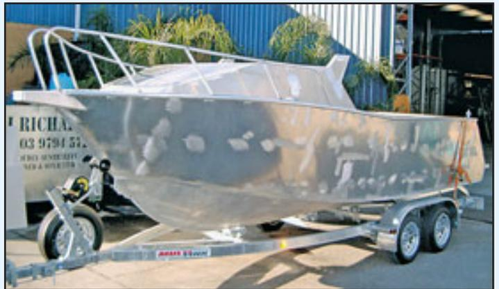
Bow rails; decide the style and fit them to the boat. Also grab rails and rocket launcher, if you plan an alloy unit, now is the time for the brackets. All of these ancillary parts must be thought of and brackets welded before the paint is applied, otherwise it will be re-work.
