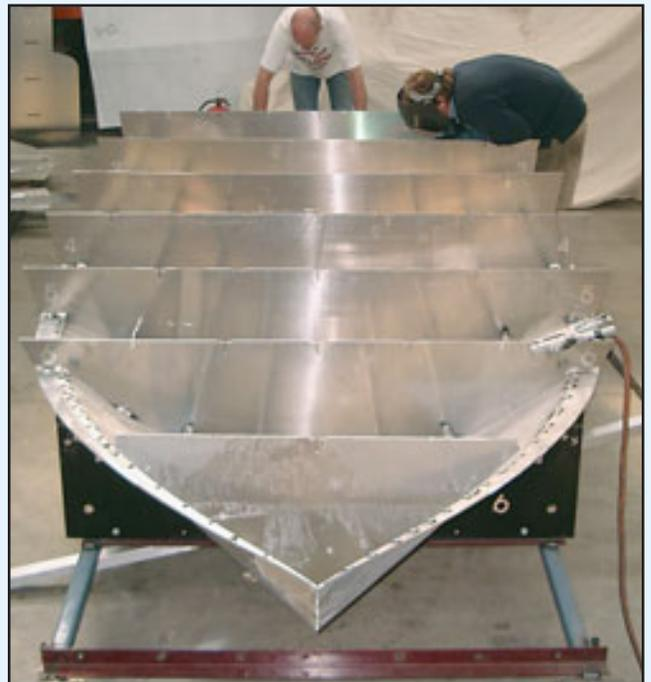
Fit the stringers and tack all plates into place. We recommend to tack weld the entire boat together, this way distortion (due to excessive heat) is minimized.
