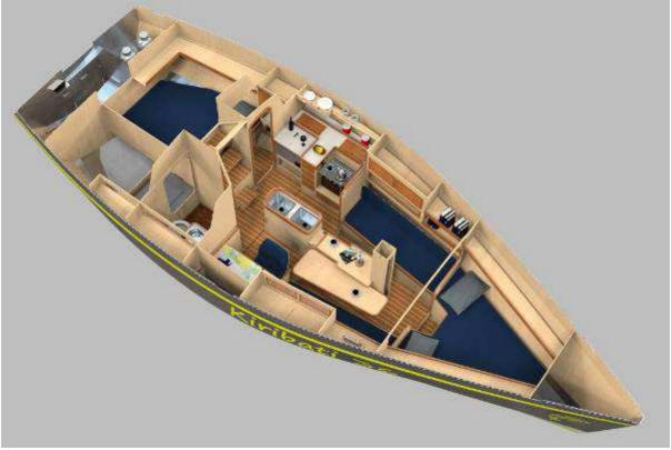
The arrangement is conceived for a couple to live aboard full time with plenty of comfort, either in port, or during extended ocean passages, having accommodations for up to four eventual guests.
