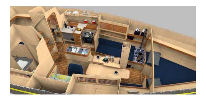
Another area seldom found on boats of the same size is the one just aft of the heads, designated as the boat's technical area, where most through-hull fittings, engine exhaust, autopilot pumps, water-makers and such are to be located. To open a main saloon locker and find the water-maker pump is all too frequent in boats that do not have dedicated areas planned for these items.
